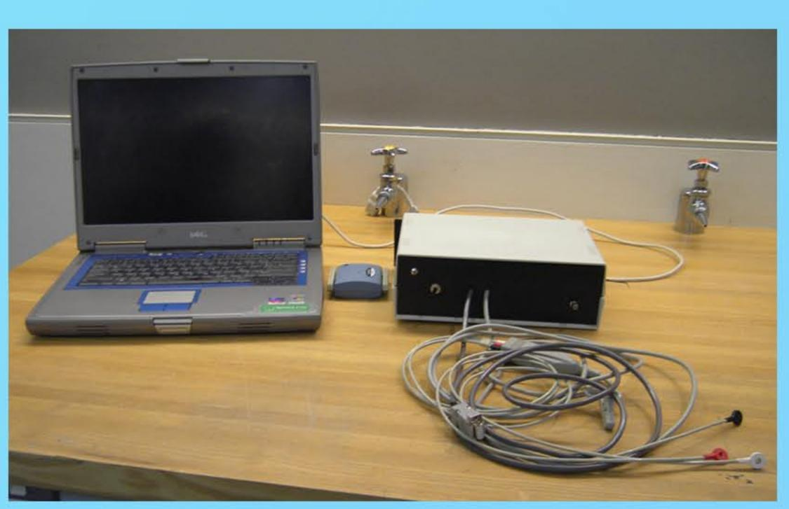
Figure 3: The set up of the previous and new device. Note the elimination of the lapto from the previous design. The laptop is replaced by a data logger that immediately stores the data output from the circuit.
