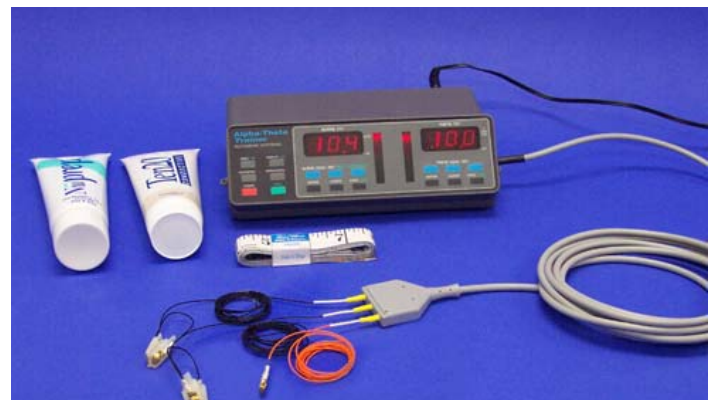
Fig. 2 – Commercially available EEG monitor; built-in theta/alpha differentiation display. This unit costs $1500.
