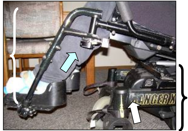
Figure 3. Photo of the user's wheelchair; the stationary base is signified by the black bracket and the tilting seat by the white bracket. The only location that would support a wrap-around bracket is denoted by the white arrow. The point of rotation for the chair's footrests is illustrated by the light blue arrow.
