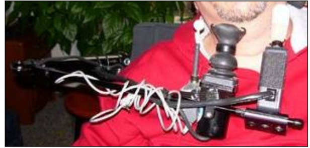
Figure 2. Photograph of the user's control bar that currently has his chin joystick (left) and tilt control (right) installed within the optimal range for use.
