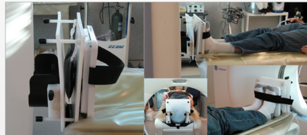
Pictures of the device attached to a GE CT table. The device loads the feet via a pneumatic mechanism that pushes a plate against them.
