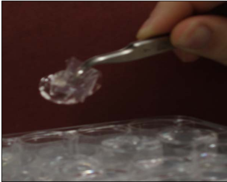
Figure 8: Hydrogel formation around a piece of PVC.
