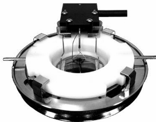
Figure 1: Bioptechs FSC® Imaging Chamber http://www.asiimaging.com/bioptechs.html
