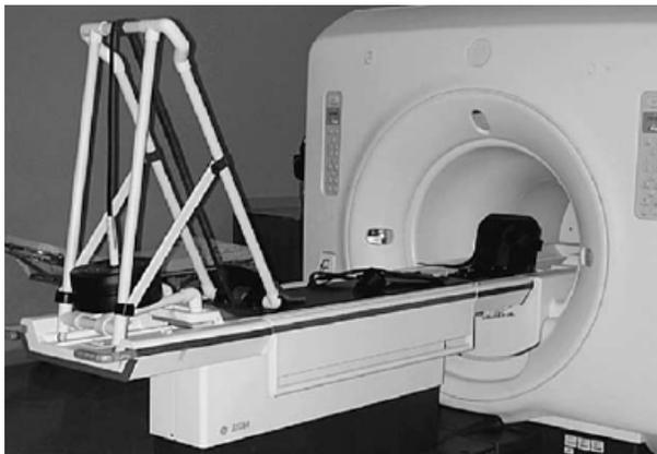
**Figure 4:** *Weight Bearing Apparatus.* Subject lies supine flexing against a constant weight of 133N. [14]
