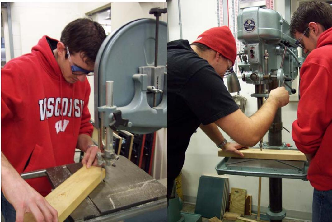
**Figure 12: Manufacturing Pictures:** A variety of machines were used to make our device such as a band saw and drill press.
