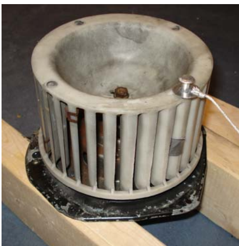
Figure 7: Fan Motor Bolt, washer, and string attached through outer rim of fan
