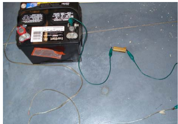
Figure 6: Battery and Power Resistor in Series
