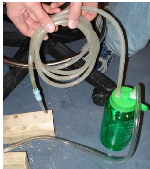
Figure 9: Collection Chamber, Tubing, and Autoclavable Tip
