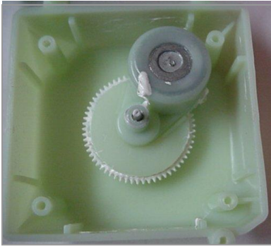
Figure 16. Off-center weight powered by gear and motor. Setup creates a vibration that can be adjusted for strength and displacement amounts (electronics.howstuffworks.com)
