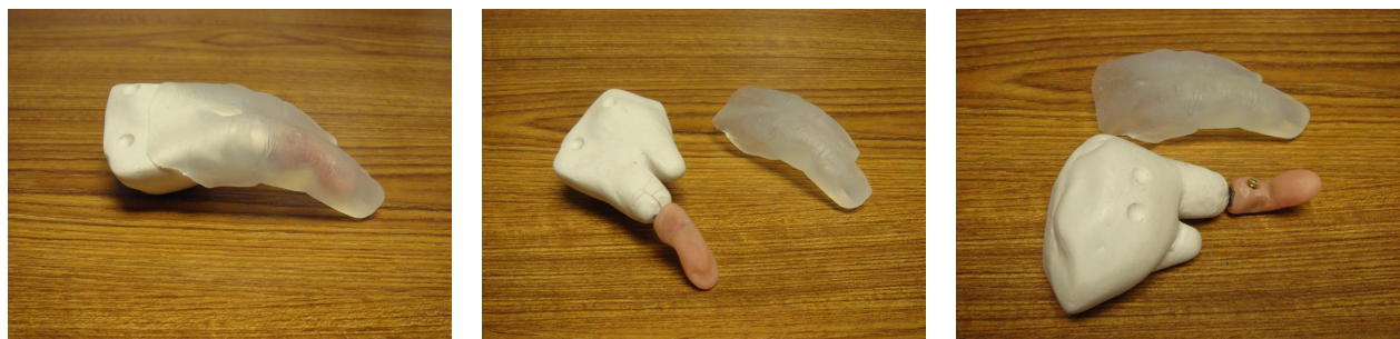
Figure 12: Final Prototype: Side View ( left ), Silicone Casting Removed ( center ), Exposed Allen Wrench ( right )
