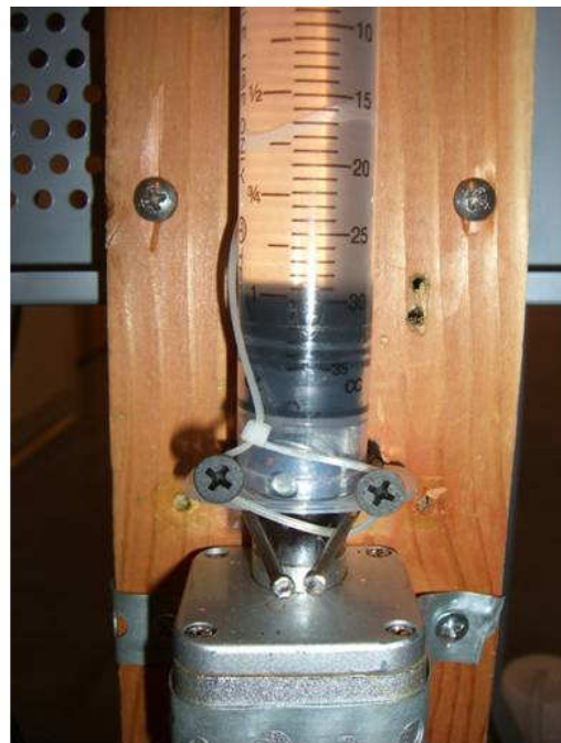
Figure 6. The actuator-syringe junction. Note the double-gasket to aid in sealing the chamber under high pressure.
