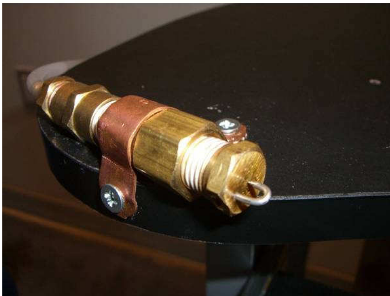
Figure 9. The spray nozzle connected to the workstation that atomizes the ethanol solution.
