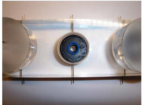
Figure 14: Assembled membrane holder positioned within lower pressure chamber. Atop the holder is an o-ring that serves to seal the membrane holder and the upper pressure chamber upon threading of the acrylic cylinder. Beneath the membrane holder is another o-ring that performs a similar function with the lower pressure chamber.
