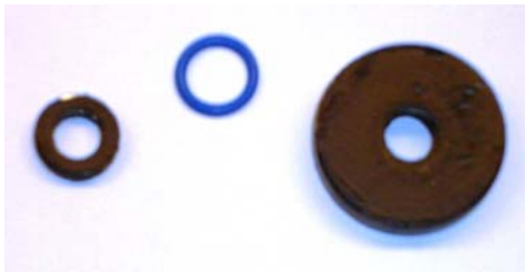
Figure 12: Components of the membrane holder, from left to right: the neodymium ring magnet, plastic o-ring, and the low-carbon steel encasing. The magnet and steel shell are coated with Plasti-Dip® rubber to prevent oxidation within the fluid system.
