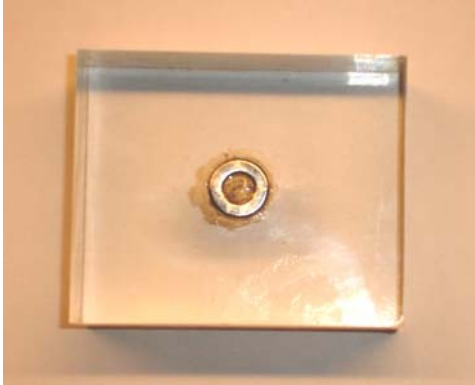
Figure 13: Loading stand for easy assembly and disassembly for the membrane holder within a sterile hood.
