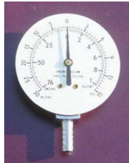
Figure 3- Frontside view of a Bourdon Gauge. (Wikipedia.org, n.d.)
