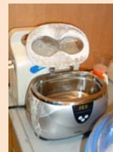
3) Sonication: removed bubbles.
