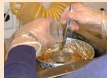
4) Spun 6g PDMS on transparency for 70 sec at 2000 rpm.
