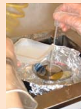
9) Added second layer of PDMS; spun for 70 sec at 2000 rpm. Cured finished sample for 20 min at 120°C.
