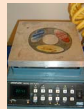
8) Cured printed sample for 5 min at 90°C.
