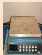
5) Partially cured PDMS for 4 min at 90°C.
