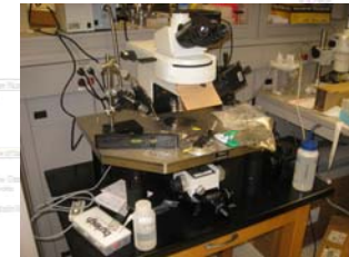
Figure 7: The location that testing is performed – a rat retina is placed on a microscope slide to record the ERG. The retina is then perfused with drugs through the liquid delivery system.
