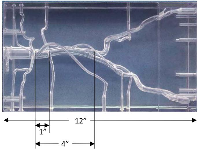
**Figure 5** - Image showing current phantom with actual measurements. This image was used to determine distance between celiac trunk, renal arteries, and femoral artery split.
