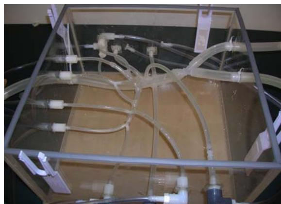
**Figure 8** - Image shows Tygon® tubing vascular network suspended within the acrylic enclosure
