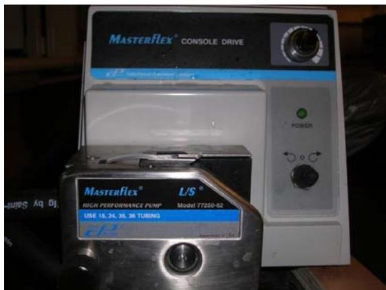
**Figure 12** - Masterflex® analog control peristaltic pump used to provide flow to the phantom
