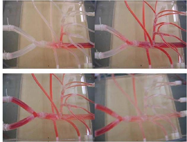
**Figure 13** – Time-lapse image of red food coloring moving through the vasculature
