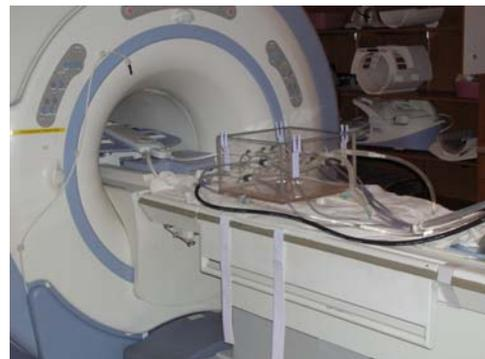
**Figure 14** – Phantom setup in the MRI scan room without the body coil
