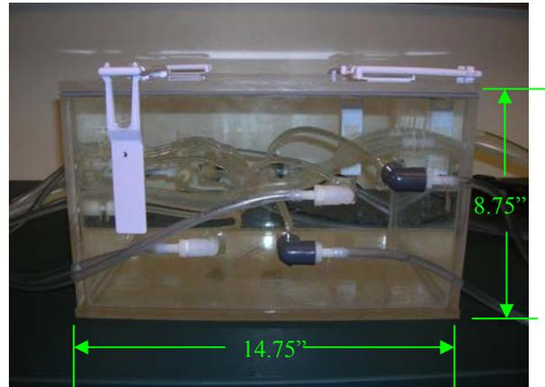
**Figure 9** - Side view of the phantom with labeled dimensions. Also visible are elbow brackets for vascular junctions exiting the side of the enclosure, and the latches use to hold down the removable top.
