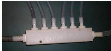
**Figure 10** - Manifold used to collect fluid from tubing within the enclosure and return fluid to the pump reservoir
