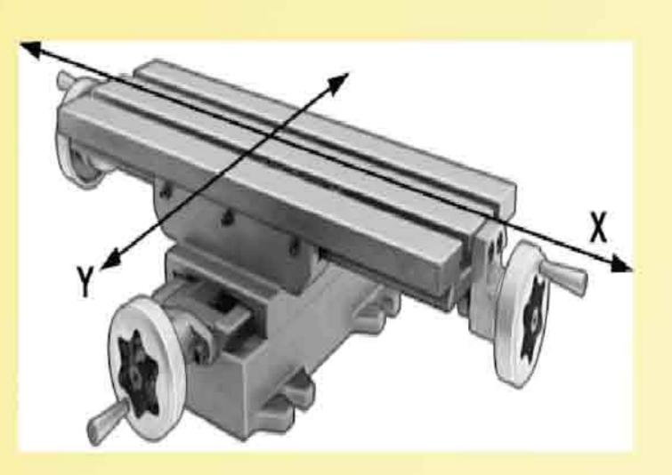
Figure 3: Fine adjust cross slide table. The handles are turned to move the table with precision 0.001m. The platform is 18" by 6", has a load capacity of 150 lbs, has a table travel distance of 12" by 8" and is 5" tall.
