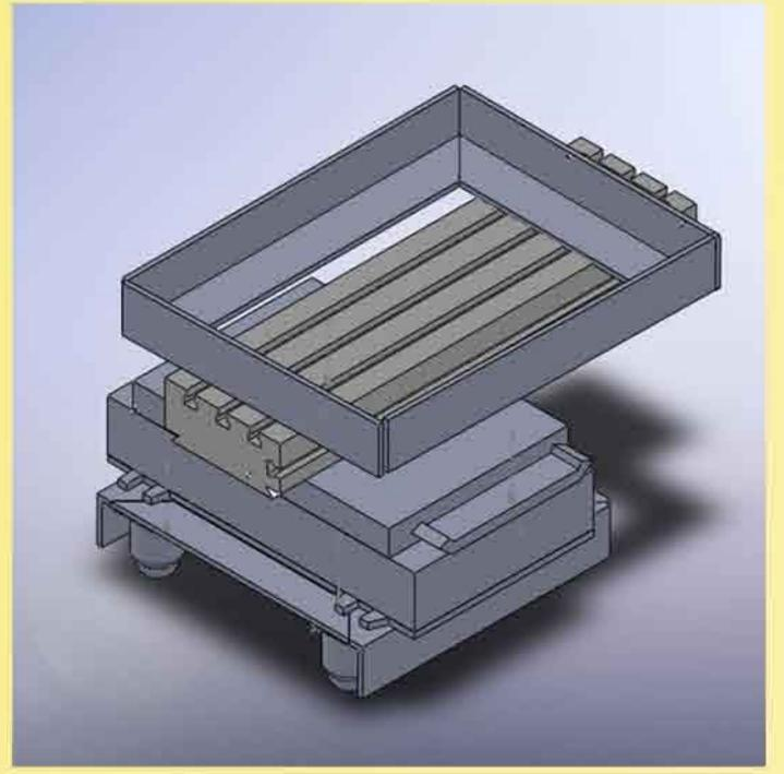
Figure 4: The complete motion stage device is shown here. The stabilizing square on top of the table holds the camera in place and is attached to the cross slide table by several large bolts. The table is then bolted to another stabilizing square. This square is shown as a cutaway in the picture in order to show the ball bearing casters. These casters allow the entire motion stage to rotate. The motion stage will sit on a table capable of motion in the z-axis.
