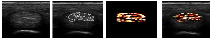
Figure 6. Ultrasound image at every step of the algorithm. From left to right: Original image, region of interest clipped out, stiffness vs. strain calculations carried out, and the stiffness vs. strain distribution overlaid on the original image. Ultrasound images provided by Dr. Kobayashi.
