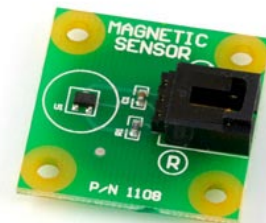
Fig. 1: Phidget 1108 Magnetic Sensor 7 The figure shows the Phidget Hall Effect sensor, which uses angle and intensity of magnetic field to determine position.
