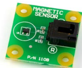
Fig. 1: Phidget 1108 Magnetic Sensor 3 The figure shows the Phidget Hall Effect sensor, which uses angle and intensity of magnetic field to determine position.
