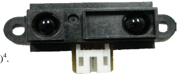
Figure 2: Sharp GP2D12 IR Range Finder 5 The Sharp infrared sensor would detect a infrared LED mounted on the surgeon's tool.
