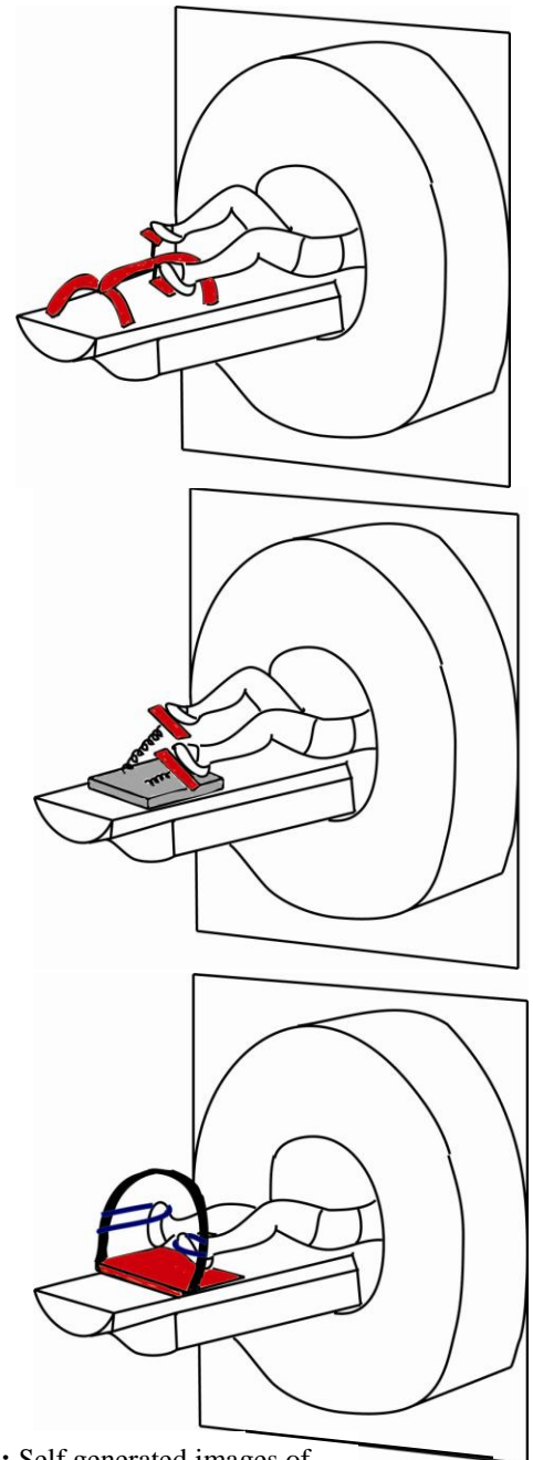
Figure 5: Self generated images of three design options. Top to bottom: Cycle, Leg Press, and Flexion.
