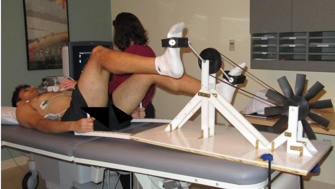
Figure 11: Team member, Val Maharaj, exercising on the cycle with Claudia Korcarz administering ultrasound scan. Notice the handles help provide stability for the patient's torso and brace the device from moving away.
