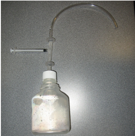
Figure 9: Prototype of final design (without BB) attached to a sample bottle with the same volume as the liquid nevirapine medicine bottle.
