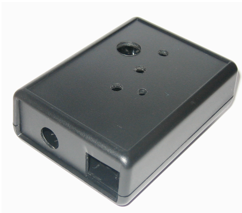
Figure 13 - The two-part ABS casing with various holes drilled for design components
