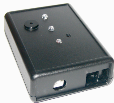
Figure 6 – The electric LED time indicator consists of three LEDs (green, yellow and red – top to bottom) that turn on at different time intervals, a recessed reset button and a speaker
