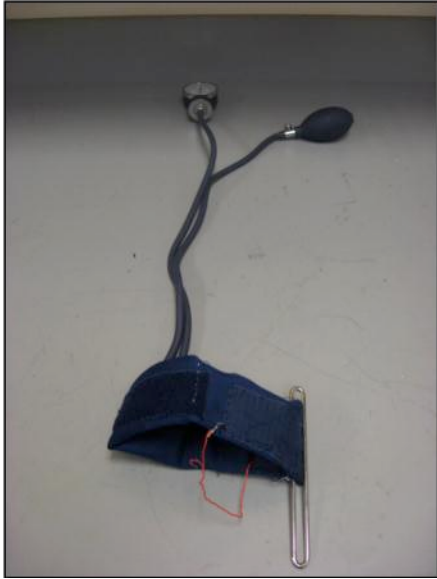
Figure 7: The modified blood pressure cuff used for the wrist
