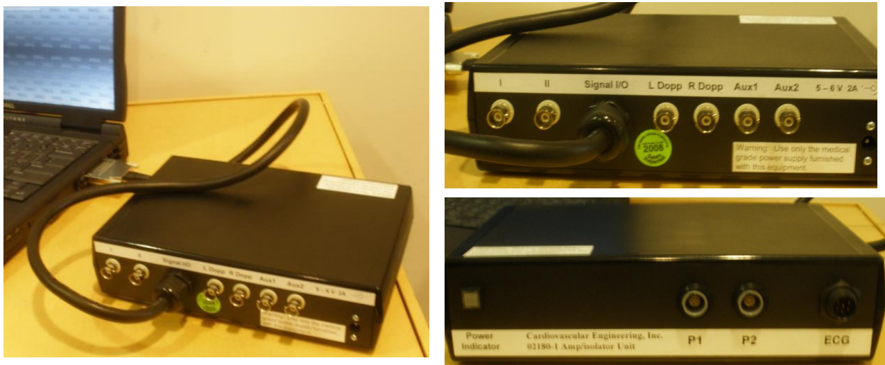
Figure 3: Depicted here are several views of the current device. Shown on the left is the current device connected to its PC with a data acquisition card. At the top-right is the front view and the back view is shown in the bottom-right.
