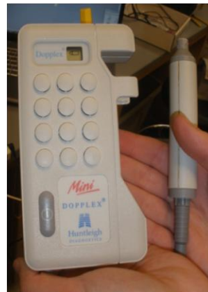
Figure 8: Mini Dopplex ultrasound transducer with an emission frequency of 8 MHz.
