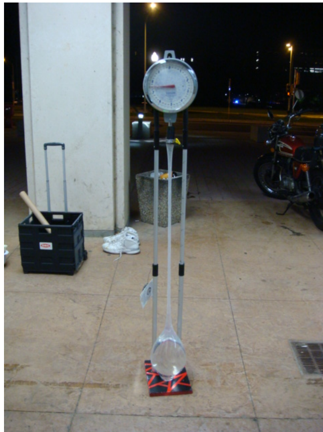
Figure 5: Water testing on the current model. Above is the old design model performing the water test. The condom was filled with water which stretched the condom to the ground and ballooned the tip of the condom.
