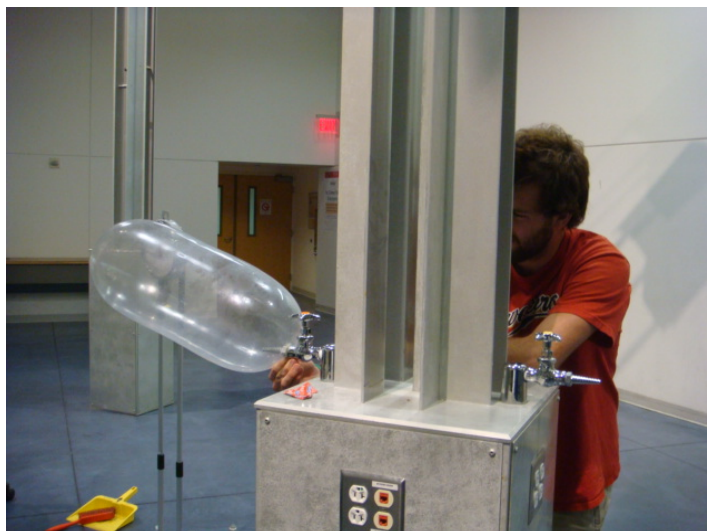
Figure 4: Air burst testing. Bret is performing the airburst test. The only compressed air we had access to was a valve attached to a lighting system in the Engineering Centers Building at UW-Madison. Bret had to hold the condom tight to the valve until it burst.
