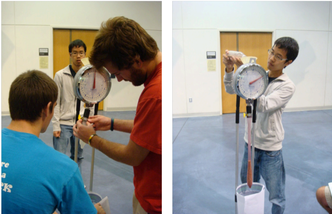
Figure 2. Testing on original model using beads. On the left, Bret is placing a condom on the old device while the group watches. On the right, Albert is pouring the medal beads into the device. The condom is stretching as the weight of the beads increases.
