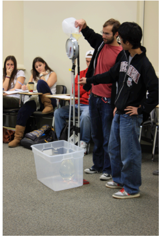
Figure 6. Demonstration in client's class. Two students volunteered for performing the condom testing. One used the beads mechanism (left) and one used the water as the testing source (right).
