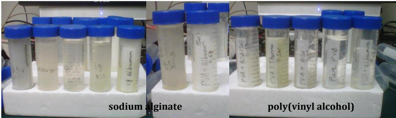
**Figure 10: Poly(vinyl alcohol) and sodium alginate gels were also tested.**
