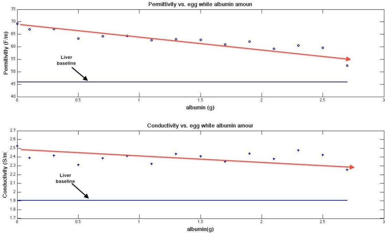
Figure 3: Adding egg white albumin lowers dielectric properties at microwave frequency (2.45 GHz)
