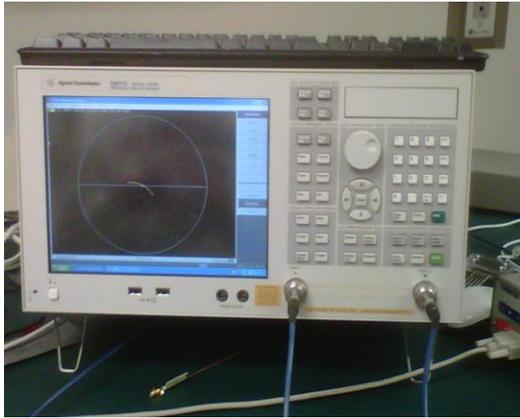
**Figure 8:** Agilent Technologies® E50701C ENA Series Network Analyzer was used to measure dielectric properties.
