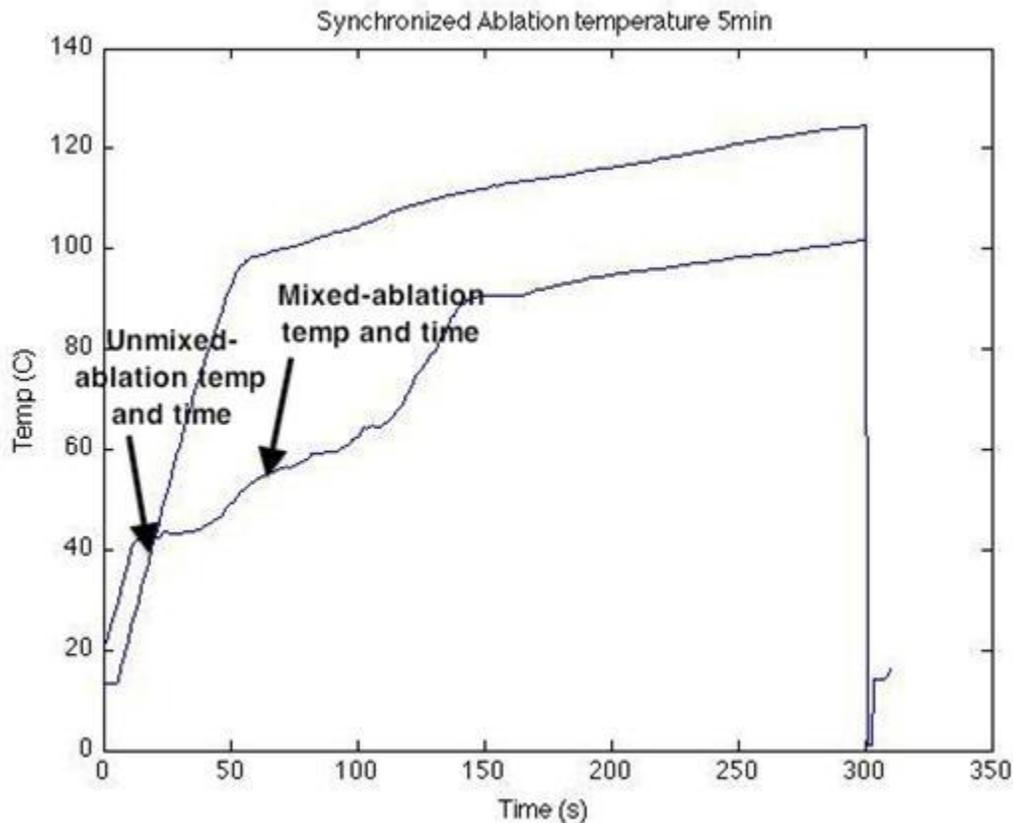
Figure 6: Synchronized temperature during ablation of mixed and unmixed egg white samples.
