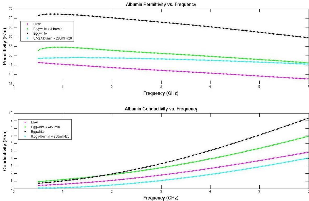
Figure 4: Comparison of dielectric properties of liver, egg white, albumin, and phantom
