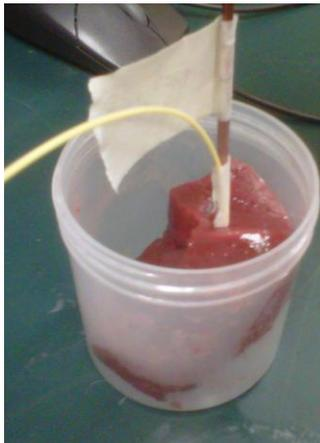
**Figure 9:** Small sections of liver were ablated for 5 minutes to determine the size of the ablation zone. The temperature probes (yellow wire) as well as the copper antenna are inserted into the liver.
