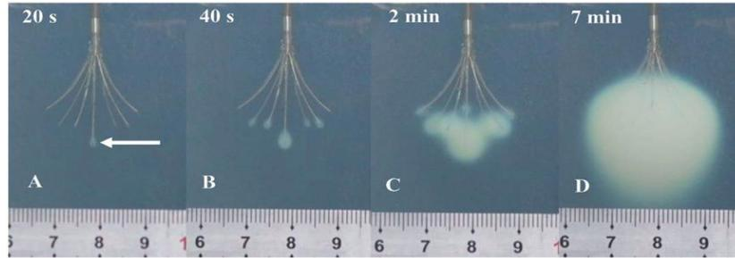
**Figure 2: Photos of ablation zones over time in polyacrylamide gel phantom and radiofrequency ablation<sup>4</sup>.**
