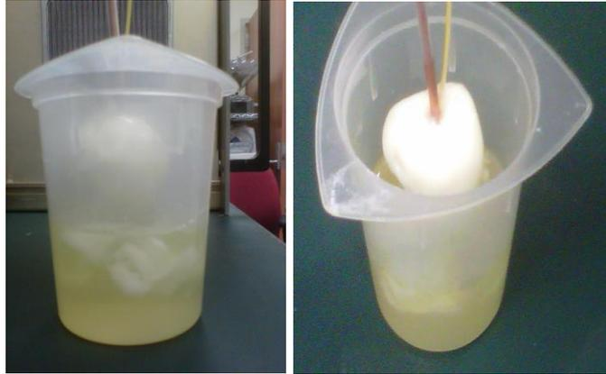
**Figure 9:** Ablation zone is clearly visible for ablated egg white. Measurements can easily be taken by lifting antenna.
