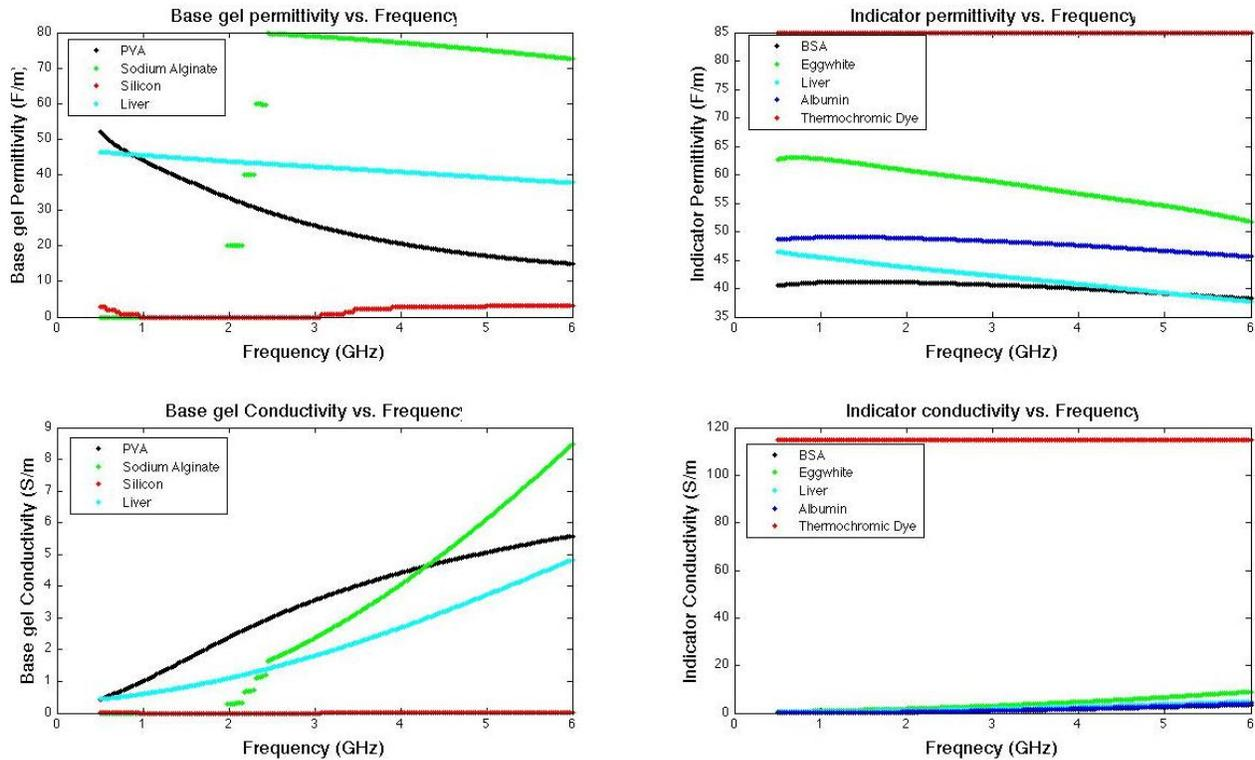
**Figure 5: Summary of dielectric properties of each base gel and indicator samples**
