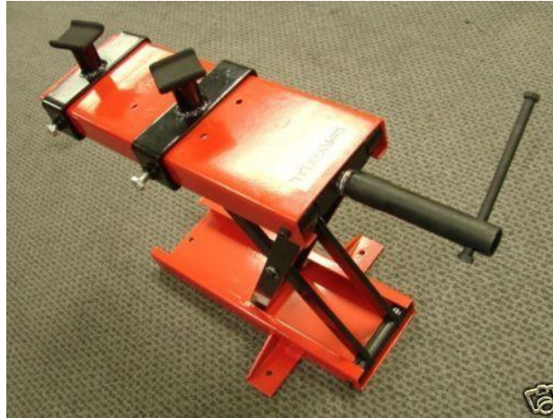
Figure 15: Motorcycle scissor jack used for vertical translation ( 1100LB Motorcycle Center Scissor Jack Lift Stand Plate, 2010 ).
