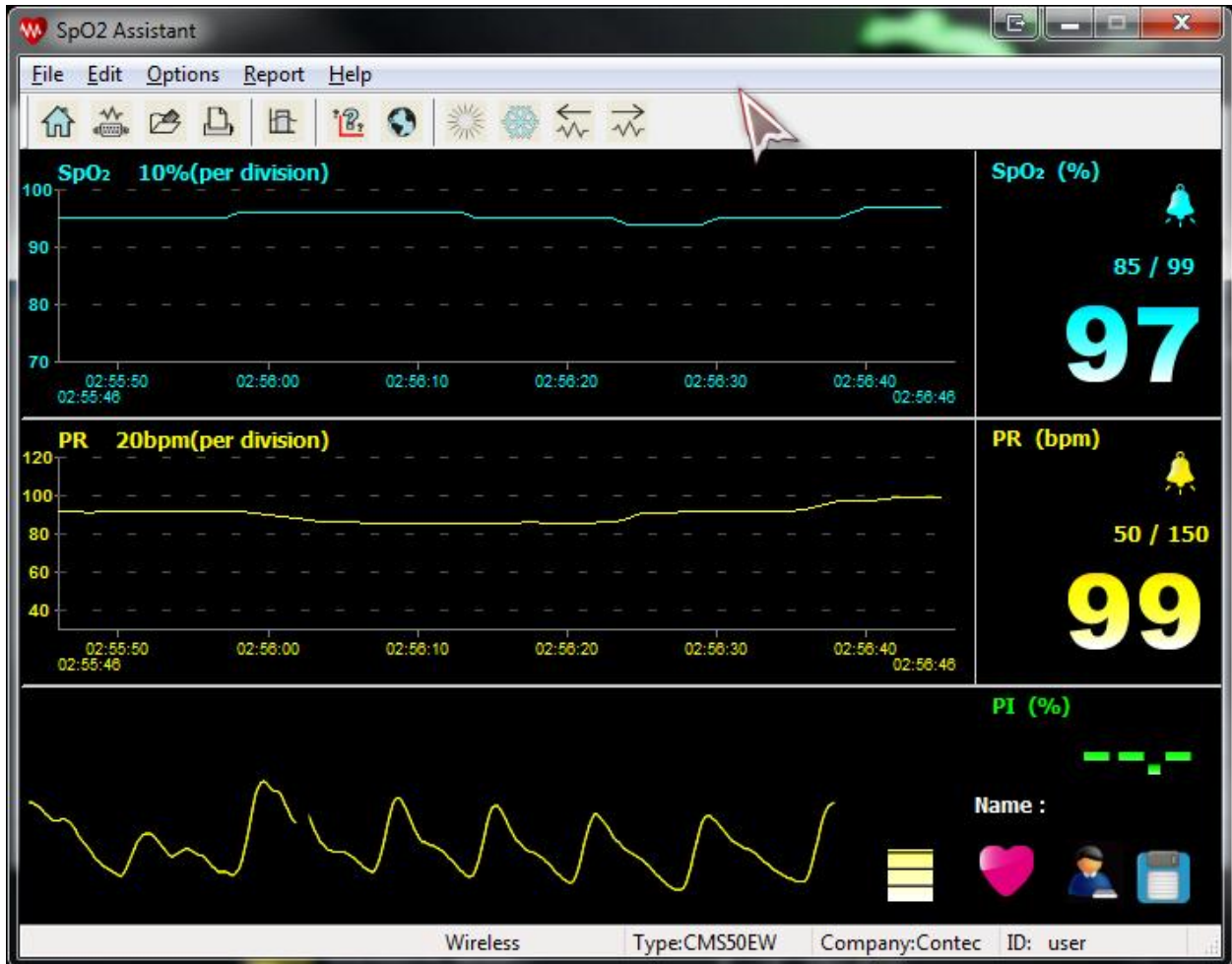
Figure 7: SpO 2 software that came with the device. Data is recorded and plotted in real time
