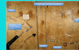
Figure 9: The lower Rube Goldberg was modified to ensure modified to ensure marbles didn't bounce off. Future improvements involve making sturdier components.
