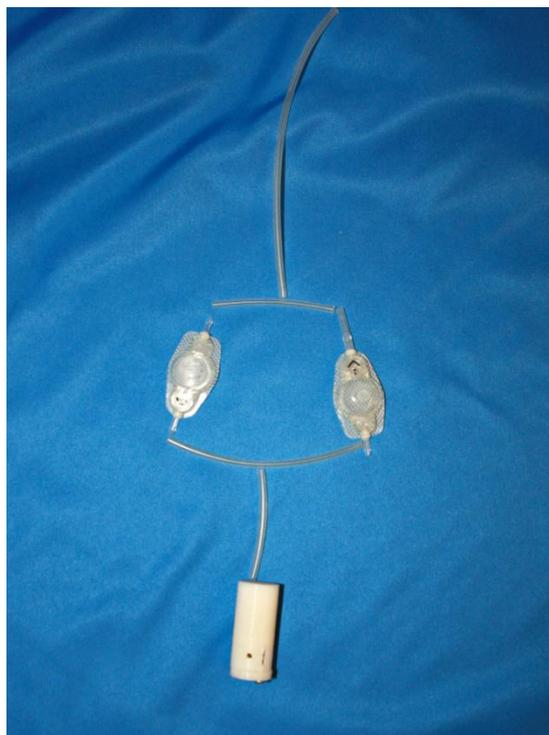
Figure 1. The setup of our system utilizing a feedback loop with a novel valve and two pressure differential valves.
