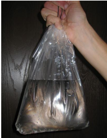
Figure 28: Seal on bag is watertight
