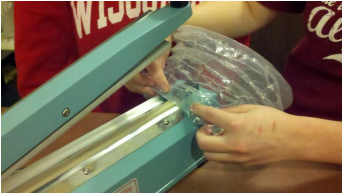
Figure 15: Impulse heat sealer creating seal on inside of accordion ring
