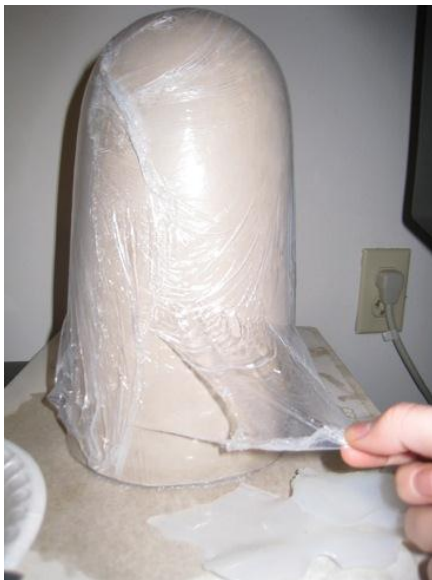
Figure 16: Clay mold used to mold EcoFlex bag
