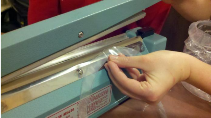
Figure 14: Impulse heat sealer creating seal on edge of accordion ring
