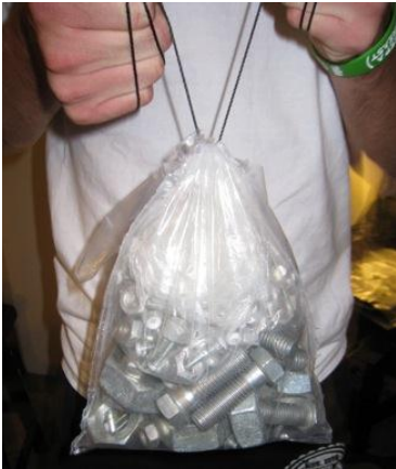
Figure 27: Testing strength of seal by incrementally adding weight in the form of metal
