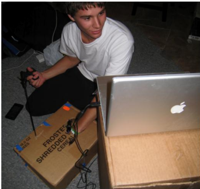
Figure 26: Josh handling a pair of graspers and using a hand to remove kidney from model abdomen while using web cam as laparoscopic element
