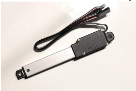
Figure 6: Linear Servomotor from Firgelli Technologies Inc. This motor is 16mm in width, the stroke length is 140mm, and the maximum force generated is 30N. Retrieved from www.firgelli.com
