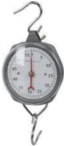
Figure 2. Above is an example of a spring in use to give a force in pounds.
