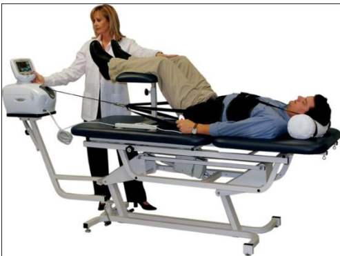
Figure 1: A traction device currently used for cervical and lumbar traction in a clinical setting. The patient is strapped onto a two-piece table that separates, applying a specific and controlled distraction force to the vertebrae [3].
