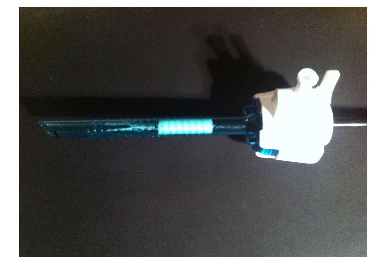
Figure 6: Snap clamp design entering trocar
