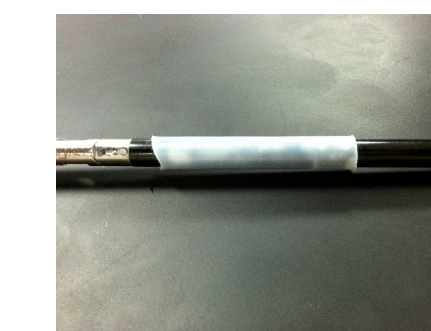
Figure 7: Applied heat shrink wrap
