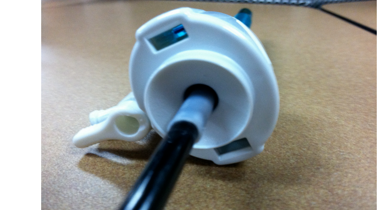
Figure 8: Heat shrink wrap design entering trocar
