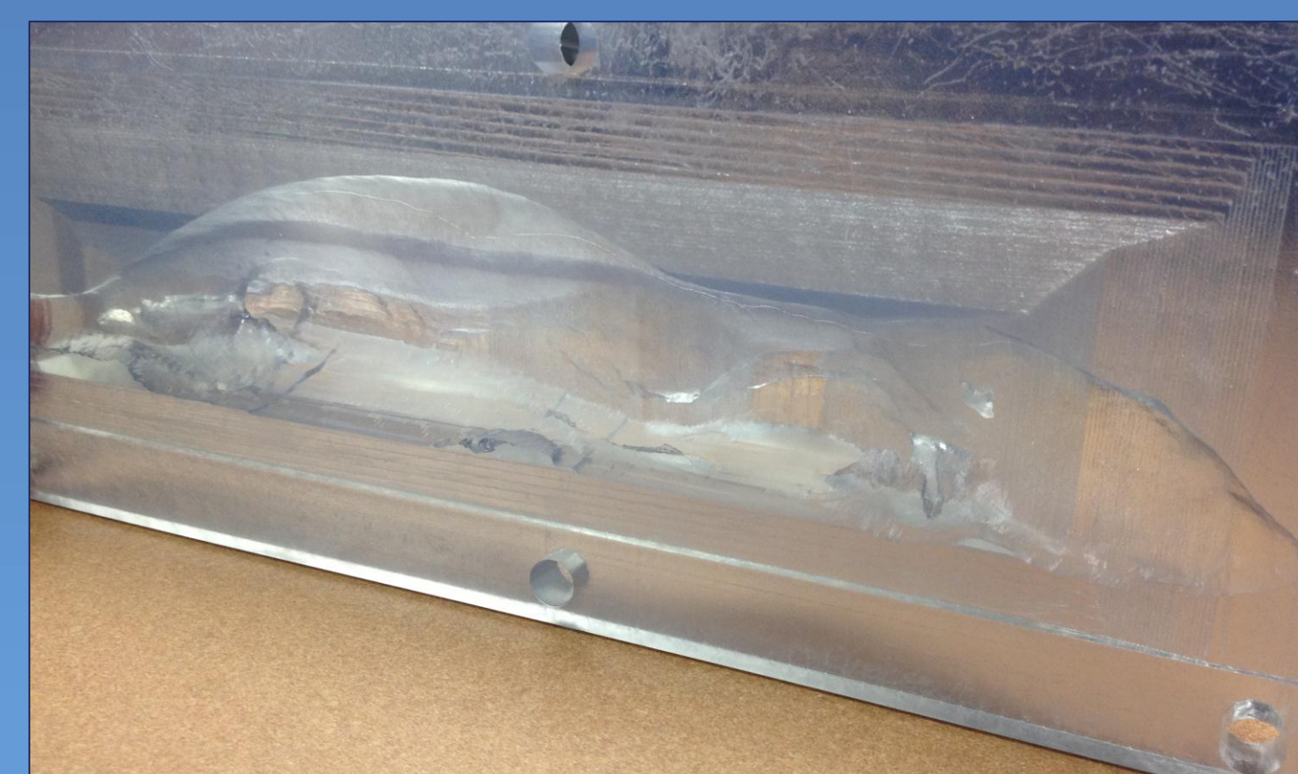
Figure 5. Negative mold of phantom
