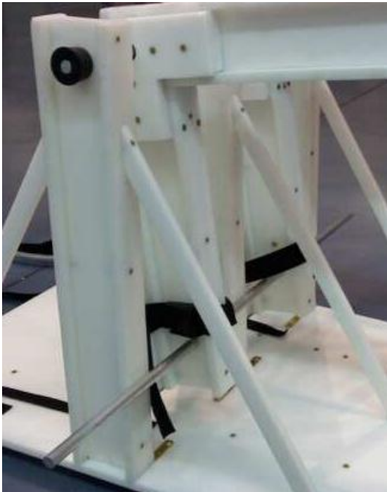
Figure 17: Stopping mechanism for the lever arms
