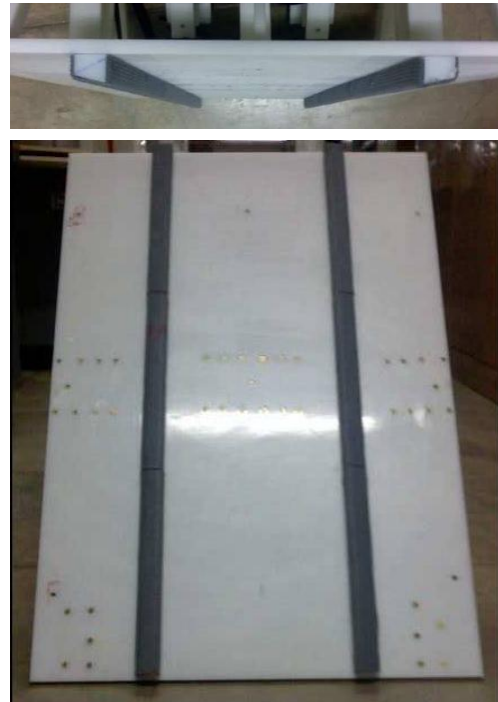
Figure 18: Base tracking made of HDPE cut at an 11.6° angle with added yoga mat padding
