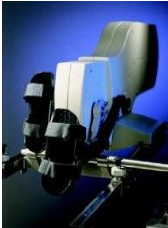
Figure 2: The Push/Pull version of the Lode B.V. MRI Ergometer [3]
