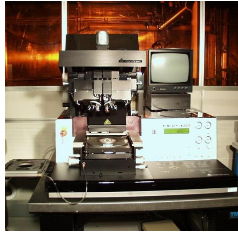
Figure 3: Karl Suss MA6 mask aligner. This device is designed for high-tech professional applications and includes digital toggles and a visual monitor. [5]
