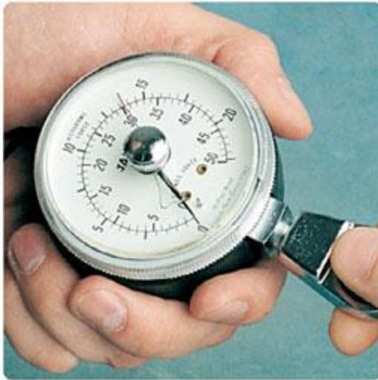
Figure 3. Jamar hydraulic pinch gauge. www.pattersonmedical.com
