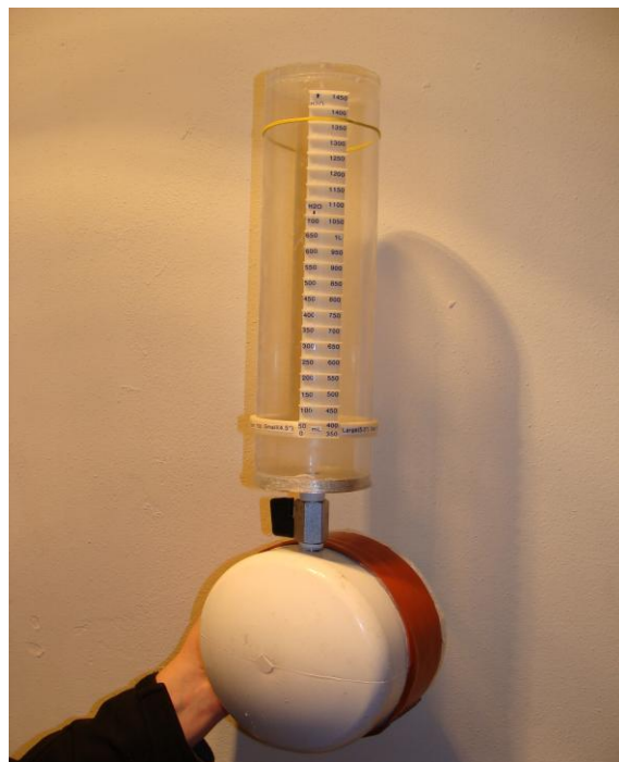
Figure 5: The final prototype with the scale for the small primary container (left) and large primary container (right).
