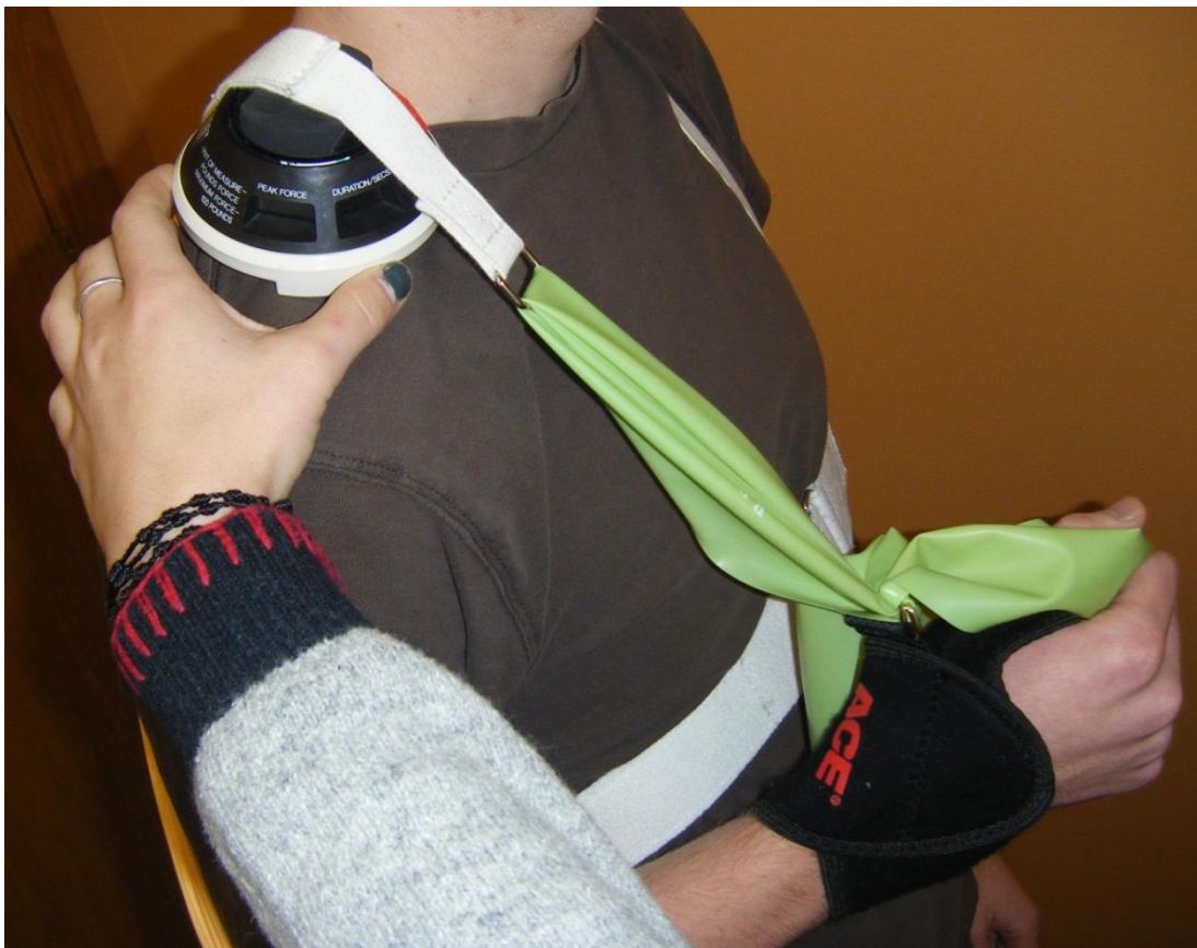
Figure 15: Testing set up as described in the body of the paper. One team member held the dynamometer in place on the user's shoulder while the user jogged in place.
