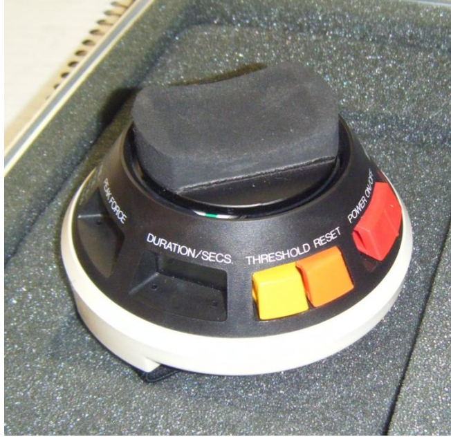
Figure 14: Dynamometer used for applied force testing. Force applied to the top is digitally displayed as the peak force.
