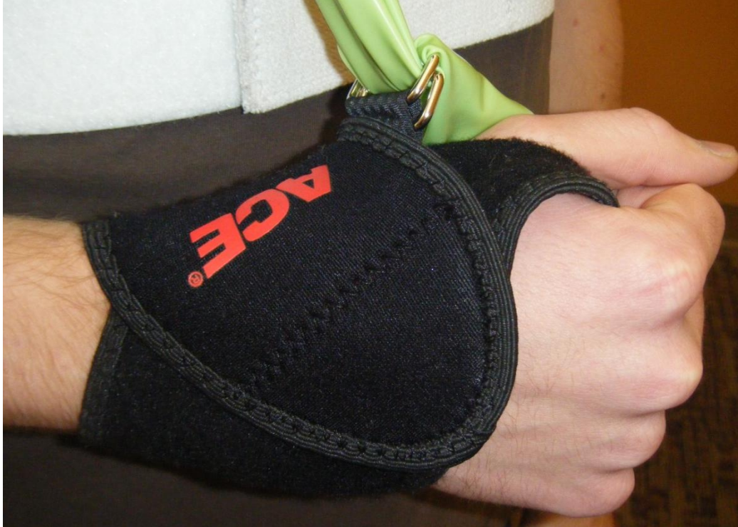
Figure 11: Wrist component of final design including the dual ring connection for the Thera-Band.
