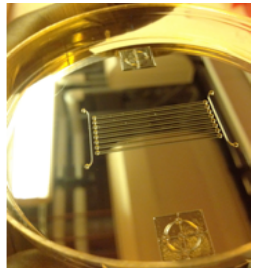
Figure 1. Master slide of microfluidic device developed by BME 301 [3].
