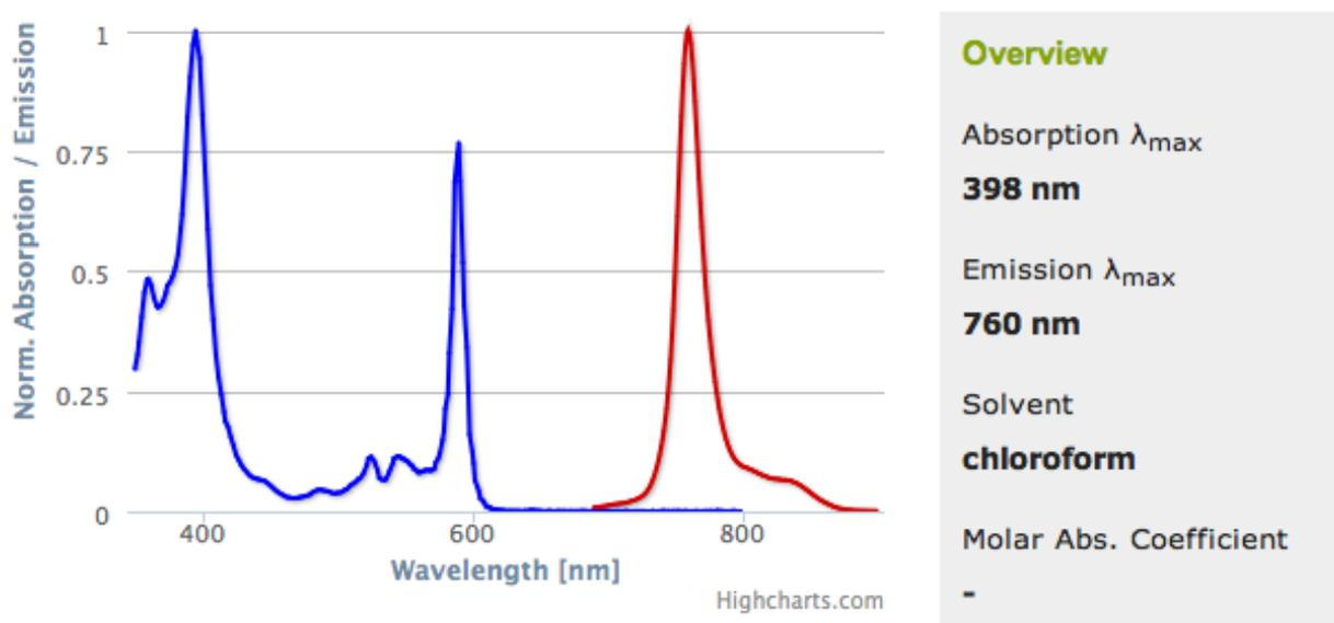
Figure 13. Absorption and emission spectra of PtOEPK [27].
