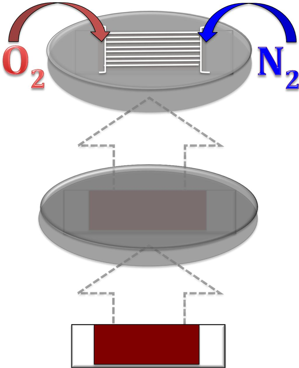
Figure 8. Thin-film oxygen sensor fabricated on a glass slide and placed beneath the microfluidic device for oxygen detection.
