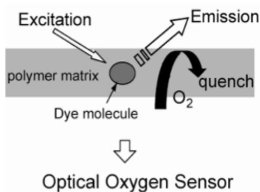
Figure 12. Diagram of how an indicator detects oxygen through an optical sensor [11].
