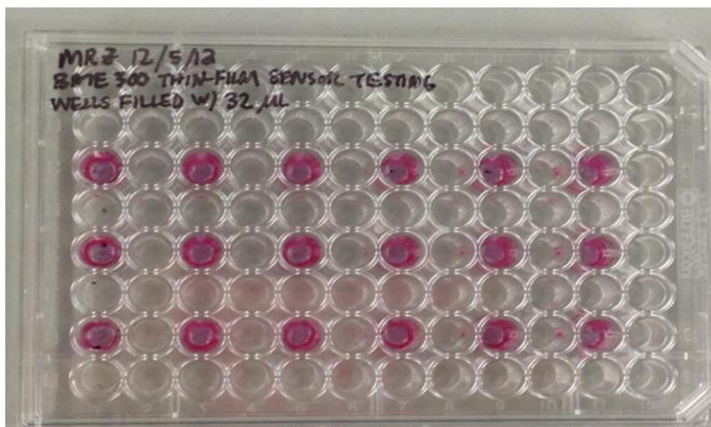
Figure 3. Placement of the final PtOEPK/PS-Toluene solution in a 96 well-plate
