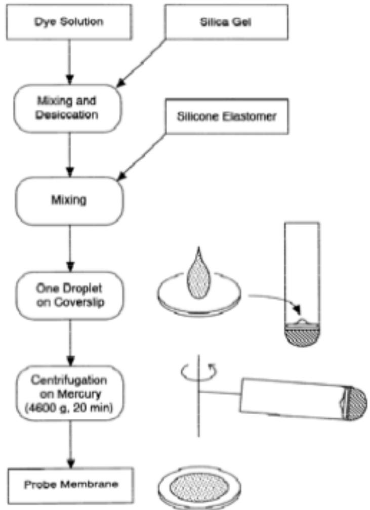
**Figure 7. Preparation of oxygen-sensitive probe membrane. This procedure yields a circular membrane that is composed of a thin layer of dyed silica gel beads and a silicon rubber film, supported by a microscope glass cover slip [13].**
