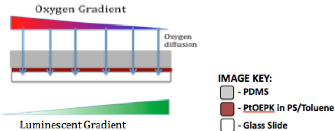
Figure 7. Slide view of thin-film sensor with microfluidic device.
