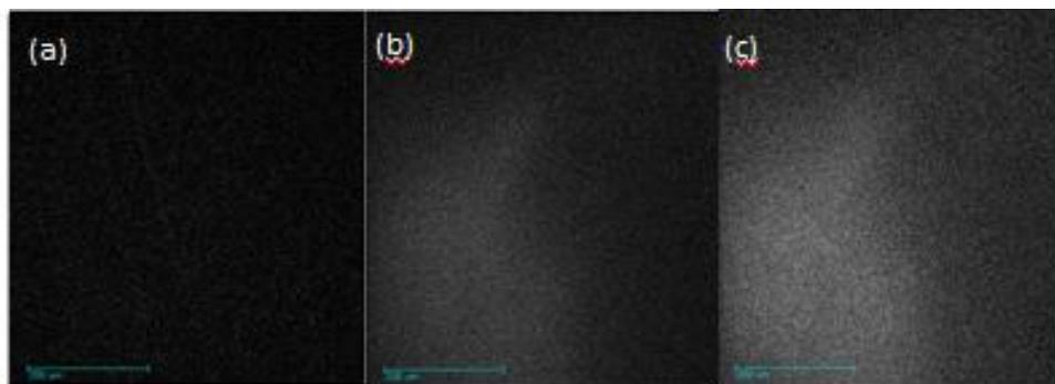
Figure 16. Fluorescent intensity of (a) an empty well, (b) a sensor well excited with a 405 nm laser, and (c) a sensor well excited with a 561 nm laser
