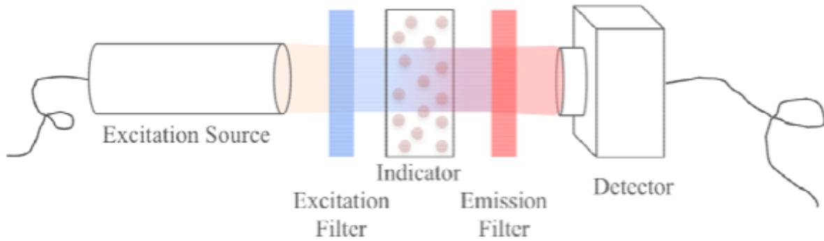
Figure 11. Simplified luminescent imaging system for oxygen sensing used for excitation of indicator material [2]
