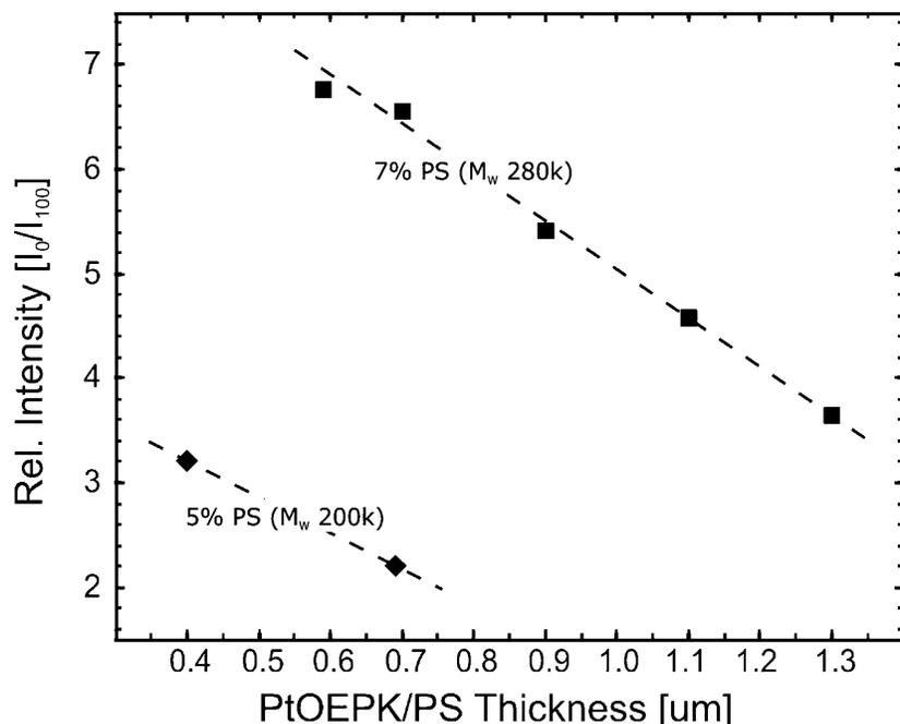
**Figure 14.** Plot of the sensor intensity ratio vs. film thickness for the two PtOEPK/PS solutions. ( $I_0$  corresponds to 0% and  $I_{100}$  to 100% gaseous oxygen, respectively). 1 mg: 1 mL ratio of PtOEPK in encapsulation matrix was used.
