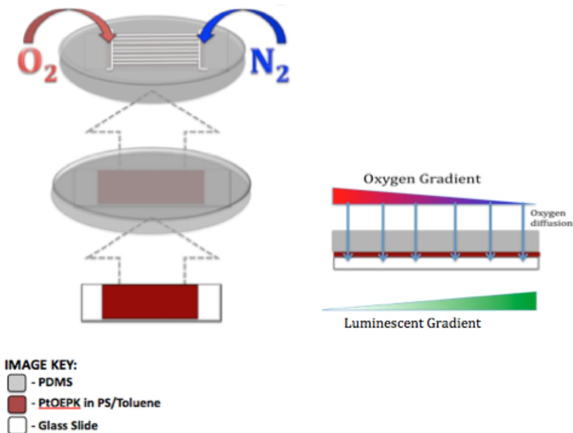
Figure 11. Thin-film oxygen sensor fabricated on a glass slide and placed beneath the microfluidic device.
