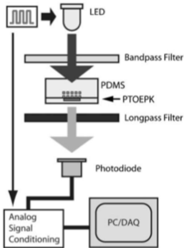
Figure 12. Optical and electrical components used in an excitation-detection system [3].
