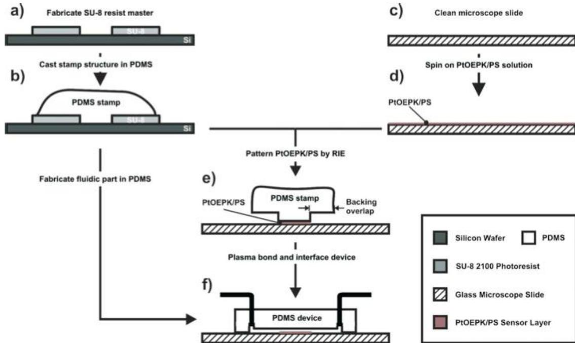
Figure 13. Schematic of the sensor fabrication process showing stamp fabrication in PDMS [4].
