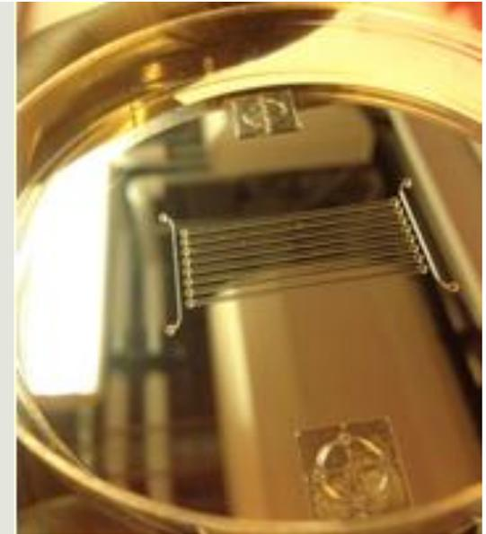
**Figure 2.** Master slide of microfluidic device developed.
