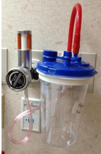
Figure 9: Photo vacuum pump used for collapse pressure testing.
