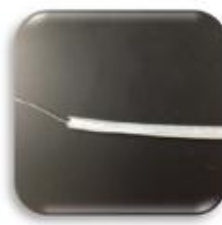
Fig 5 – The silicone tubing is cut flush with the heat shrink tubing.
