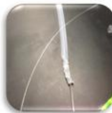
Fig 2 – Wire is wrapped around the end of the silicone tubing.
