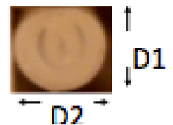
Figure 16: Cross-section of Sani-Tech® 50 sample for recovery test, demonstrating D1 and D2 measurements.
