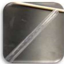
Fig 1 – Perforations are made along the length of the heat shrink tubing.
