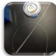
Fig 3 – Wire is anchored in the notch of one end. Half the wire is inside the heat shrink tubing and the other half remains on the outside.
