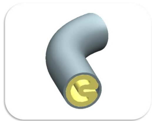
Figure 3: CAD model of the cross section of the first design alternative, showing a folding inner tube with a sleeve. (image generated by Megan Halley).
