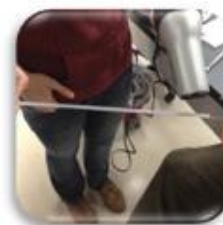
Fig 6 – A hair dryer shrinks the tubings down to collapse the silicone tubing onto itself.
