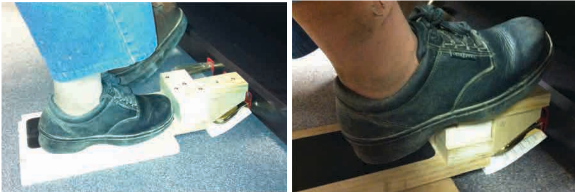
Figure 11: Prototype testing. The left side depicts the placement of the device and Mary’s foot, which resulted in discomfort for the user. The right side shows the ideal placement of the device and users foot.
