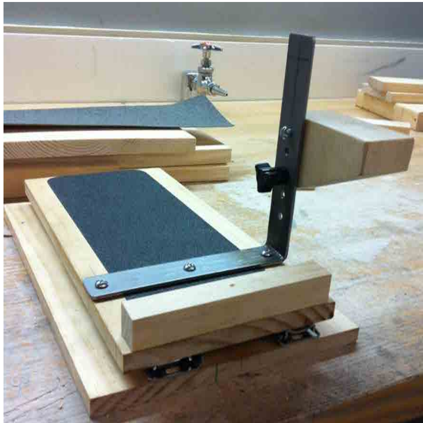
Figure 10: Final design. Gliding wedge system with adjustable height wedge.
