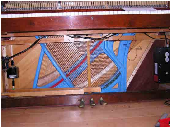
Figure 2: Components involved in the pipette design created by Michiel van Loom include a solenoid, control board, power unit, and pedal rods [4].
