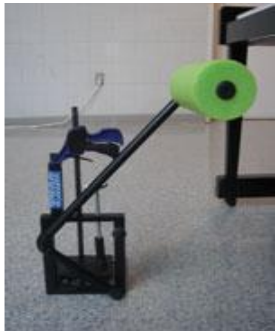
Figure 1: Thigh-controlled piano adaptation device created by Duke University [3].
