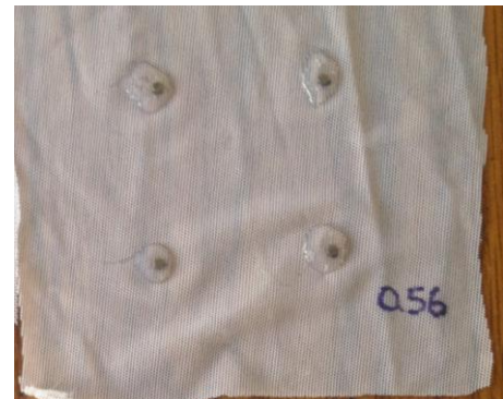
Figure 3: Four magnets (in the 1 inch x 1 inch arrangement) adhered to power mesh using silicone A-564.
