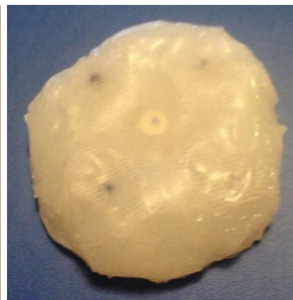
Figure 9: One of the small-scaled placenta models with the four placement magnets surrounding the sensor magnet.
