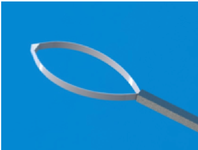
Figure A9. The original loop design worked similarly to the current clamp design, but had two equally thin steel ribbons, and a steel triangle at the end to act like a spring to push the ribbons apart, as they were pushed out of the tube. The tube as shown above was also a square instead of round.
