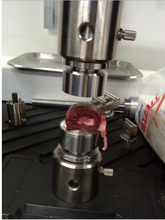
Figure A4. Porcine Kidney Compression Testing.
